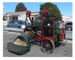
We believe it was used locally on storm water and sewer junctions and ran day and night for weeks at a time. It would have been phased out in the early 1960,s when certified premixed concrete was introduced.
